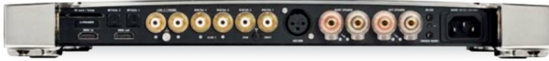
ABOVE: The amplifier is fully configurable in software [boxout, p49], all parameters loaded via an SD card slot (top left corner). The HDMI inputs are yet to be enabled
