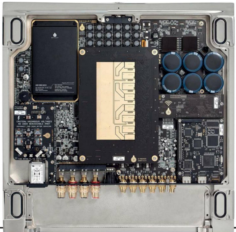
RIGHT: Exquisitely engineered, the D-Premier features a 600W switchmode/PFC PSU (top left), proprietary digital Class D current dumpers (centre) and Wi-Fi module (centre right)
